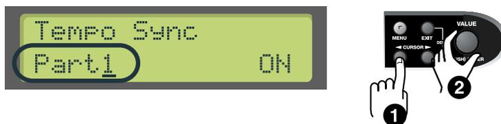
5. Use the **[CURSOR]** buttons to move the cursor to the “ON” (or OFF) location, and turn the **[VALUE]** knob to switch the setting ON/OFF.
