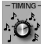
The arpeggios are synchronized to the tempo of V-Producer. This knob specifies the note value (note timing step) for each note of the arpeggiator when synchronized.
