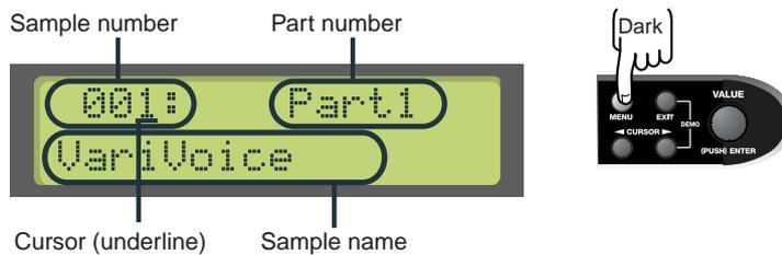
2. Make sure that the cursor is located at the sample number, and turn the **[VALUE]** knob to select the desired sample.
