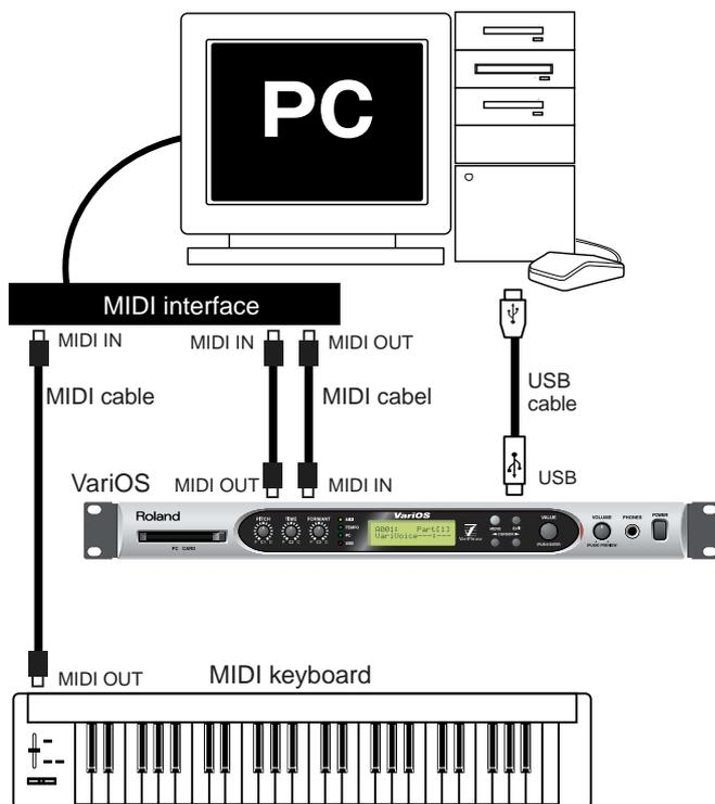
\* Since the VariOS uses the USB cable to transfer wave files from the computer, you must use a USB cable to connect the VariOS and your computer even when you are connecting to a MIDI interface.
